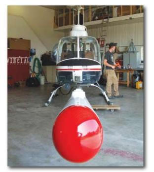
The Structural Multi-View System is certified for use on a Bell 206 Jet Ranger and Eurocopter's ASTAR AS 350. The portable package can be quickly and easily shipped to any destination utilizing local helicopters and pilots.
